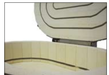
Kiln interior with circular lower side heating
