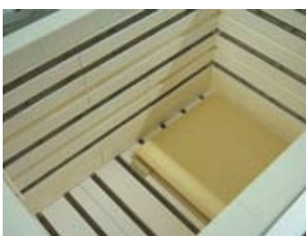
Firing chamber with heating from 5 sides
