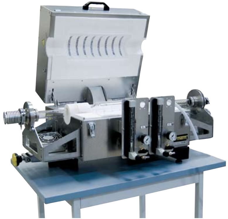
RSR 80-300/11 in tiltable version with glass tube and protective gas operation
